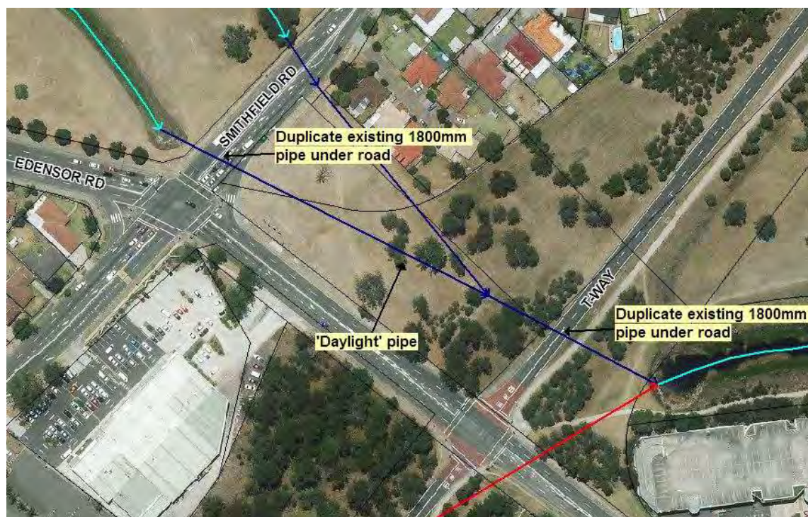
Figure 40 – Schematic plan of proposed pipe upgrade, Edensor Creek
