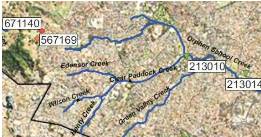
Figure 46 – Distribution of existing rain gauges and water level recorders in the Three Tributaries catchment
