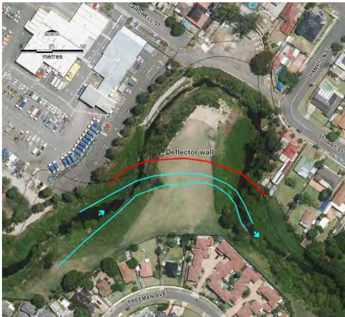
Figure 38 – Proposed channel realignment, Orphan School Creek near Freeman Avenue (after Dalland and Lucas, 1996)
