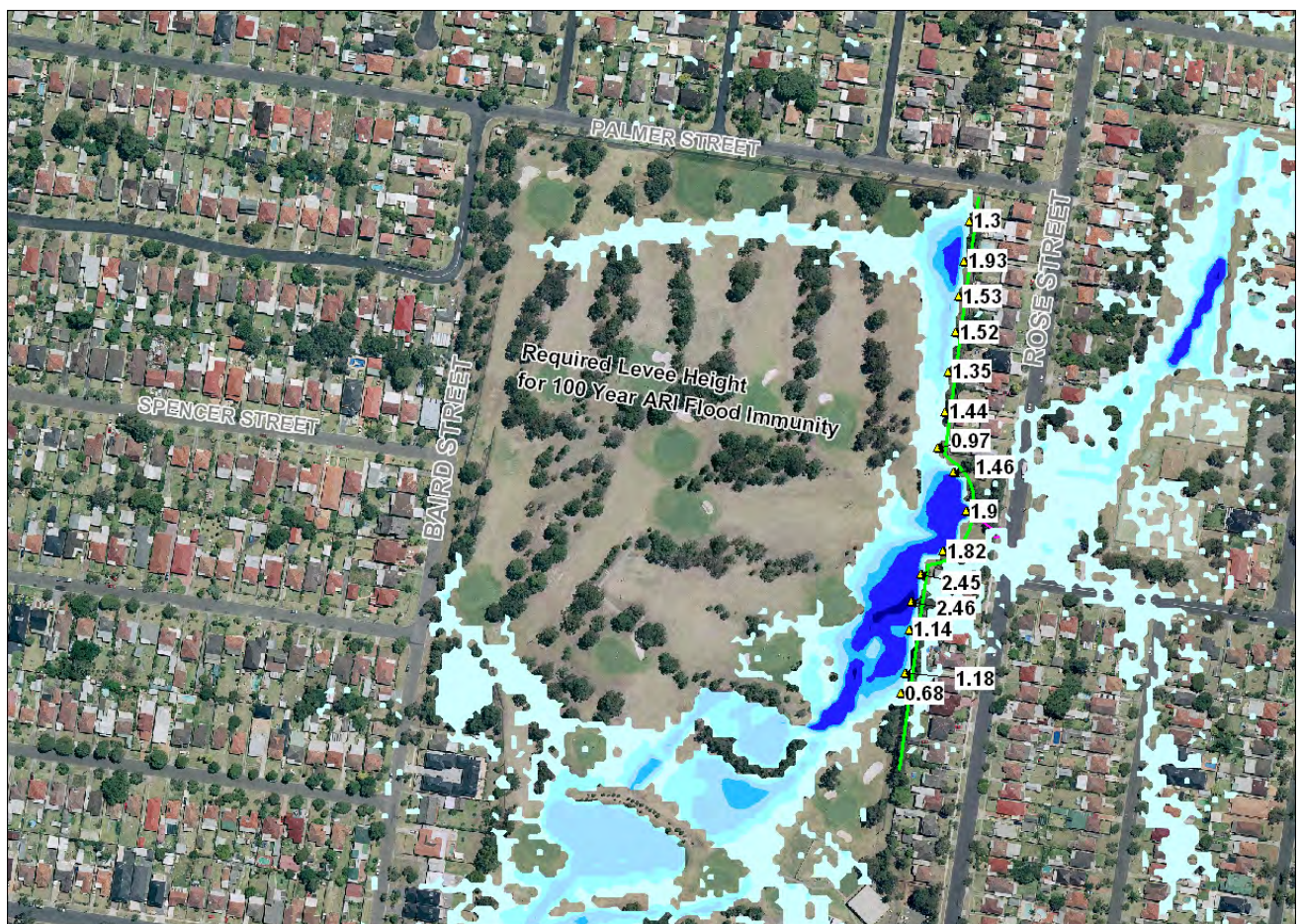
Image 6: Retention Basin Wall Heights Required To Contain The 100 Year ARI Flood
