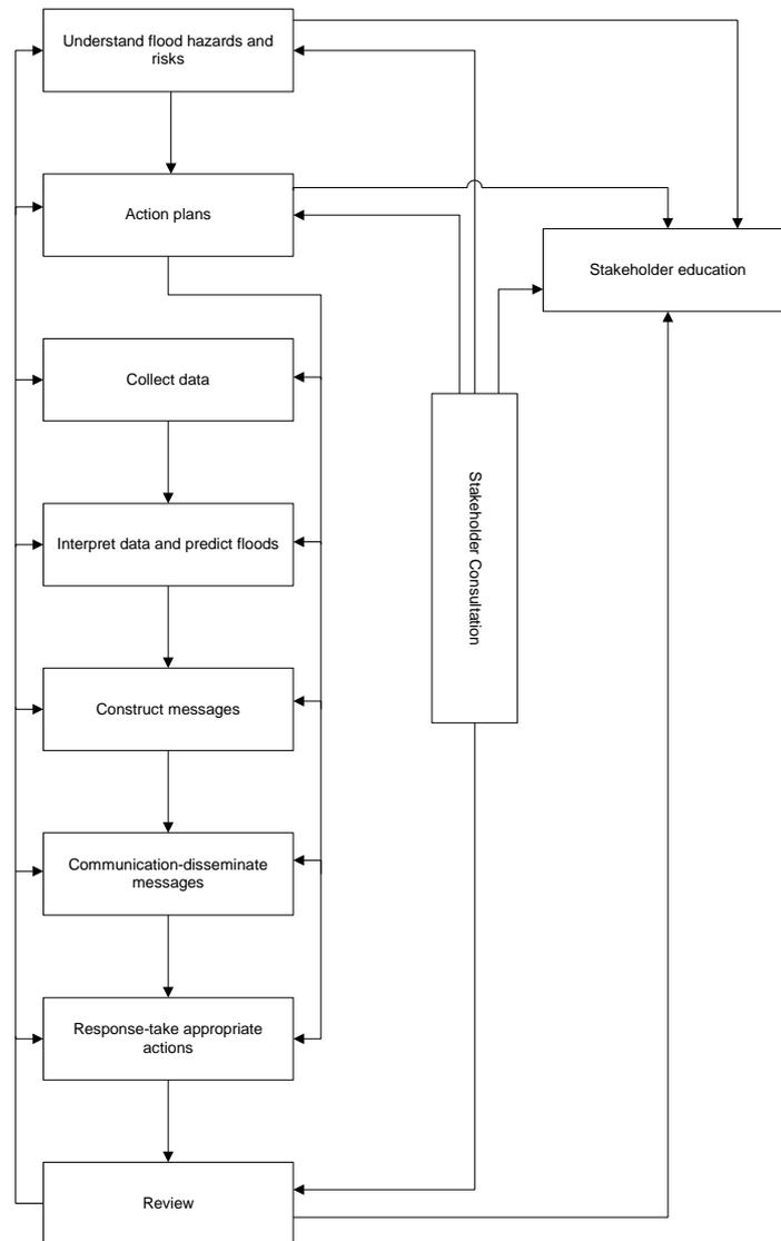
**Figure 2: Expanded TFWS components (source: Molino et al., 2011)**
