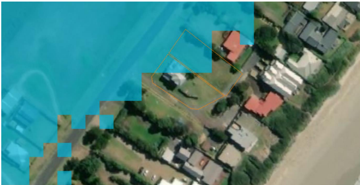
Figure 7: Isolation caused by the 1% AEP flood.
